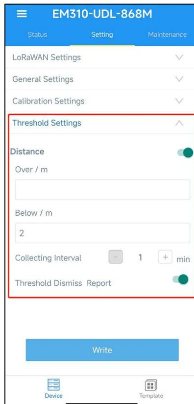
Take the configuration in the above figure as an example, here I set the "Below" option to 2 meters and then enable the “Threshold Dismiss Report” option, when a vehicle enters the corresponding parking space and the sensor detects that the distance to the object (vehicle) **is less than** 2 meters, the data will be reported. And when the vehicle leaves the corresponding parking space and the sensor detects that the distance exceeds 2 meters, the data will also be reported.
