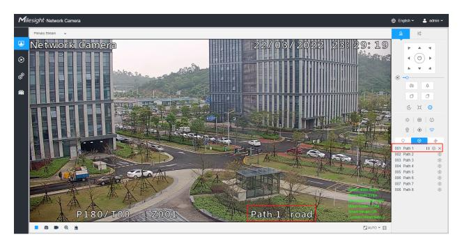
Step2: Use the PTZ control buttons to move the lens to the interested position;
