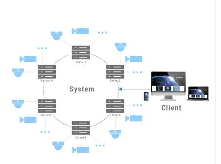
Taken over by multiple servers simultaneously. Cameras will be allocated to servers automatically to do load balancing.
