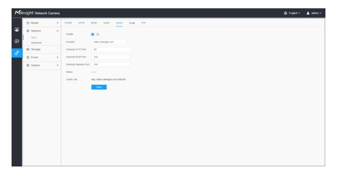
You can choose "ddns.milesight.com" as provider for DDNS. After enabling it, you can access the device via the URL "http://ddns.milesight.com/MAC address".
