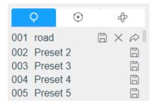
Note: The following presets are predefined with special commands. You can only call them but can't configure them. For example, preset 037 is the "Self Check". If you call the preset number 037, the PTZ camera will start self check function at once.
