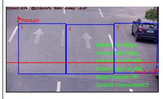
The Radar detection area is a rectangle with diagonal lines in the two coordinate points;
